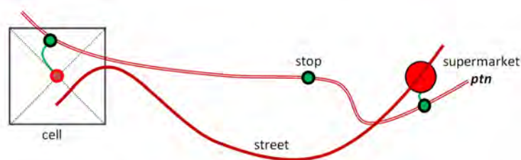
Figure 70: Depiction of the rule set for accessibility; green lines correspond to pedestrian access by using the street network.
