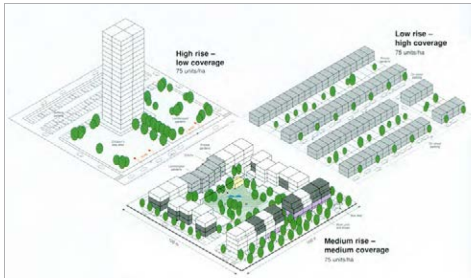
Figure 47: Relationship between built form and urban density - all building mass models cover a density of 75 units per hectare (from Rogers 1999:62).
